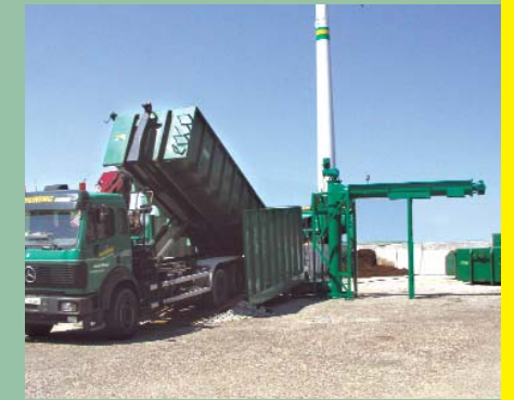
Drive-on reception station with metered screw discharge and hydraulically actuated live bottom floor
