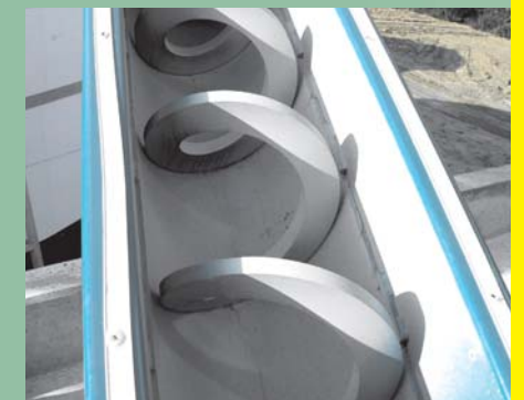
Screw conveyor system horizontal, vertical and inclined; tubeless screw
